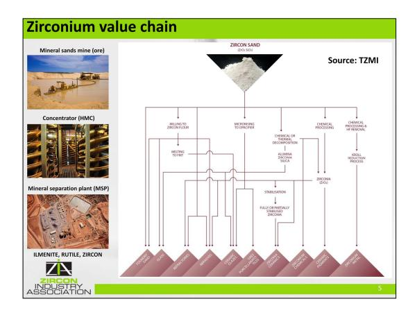
Zircon is found in so-called mineral sands, containing mainly the titanium minerals ilmenite and rutile, and zircon. Mineral sands undergo two main stages of beneficiation - first production of a heavy mineral concentrate and secondly separation into the various constituent minerals.
