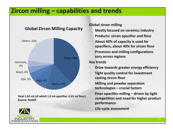
A large part of the demand for zircon from the investment casting industry is in the form of flour, so I thought that I would include some information about milling capacity here. As can be seen from the chart on the left, zircon milling capacity is of the order of 1.65 million tonnes, of which 60% is geared to production of opacifiers for the ceramics sector.
