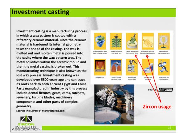
I suspect that most here are familiar with the investment casting process - for those that are not, the text on the left is a summary I found on the internet. The graphic on the right is a good pictorial representation. It is in the ceramic shell which covers the wax patterns that zircon is used.
