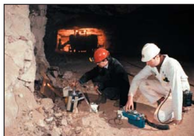
Measuring radon levels in mines
