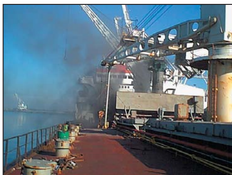
Dust generated during unloading from a ship
