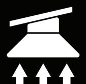
Use dust extraction systems when dry milling zircon, loading material into a processor or bagging a powdered product.
